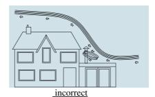
Avoid the chimney opening out onto areas near buildings, where the air may be turbulent and inconsistent.
