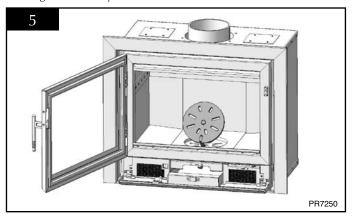
4a.2 The main grate can then be lifted by the front first and then rotating the main grate to clear the firebox.
