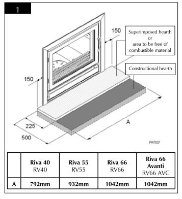
If you are fitting the Riva MF into an existing hearth setting check that it complies with the current regulations and is the minimum size shown.
