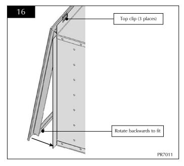
7.2 The main frame can now be by rotated into position on the front of the appliance body and fixed in place with the trim fixing screws.
