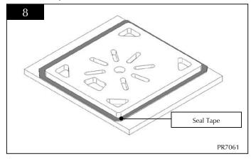
4b.5 Ensure that the grate sits flat on to the side supports, and that no debris are trapped under it. Check also that the centre grate sits flat and rotates freely with no debris trapped under it.
