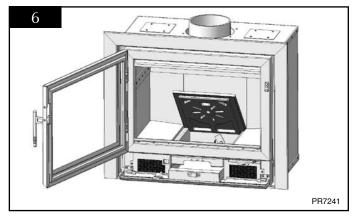
4a.3 Ensure that the seal tape on the underside of the grate is in good condition and correctly fitted. If not, replace with new. (Stovax part number 4998)
