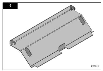
3.3 **Second** remove the **Upper Baffle**, see diagram 4, by pulling forward to disengage it from the hanging points at the top of the firebox. Rotate the baffle to remove from the firebox through the door opening.
