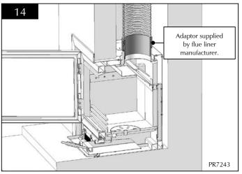
6.7 Should the Riva MF be installed on an unlined, masonry flue, first fit a non-combustible closure plate to locate the first section of single wall flue pipe from the Riva MF to the old system. Then make the connection as with a flue liner system. Do not connect the system into large voids that could exist in older chimney systems. If this is the case consider using a flue lining system to improve the Riva MF operation. See diagram 15.
