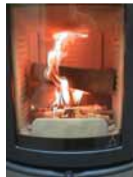
Figure 4: close the primary air
