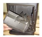
7. Remove the rear heat shield using a 10mm spanner or socket wrench
