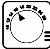
Use radiator or room thermostats to control the system, not the controls on the stove
