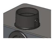
Wind the eight M6 studs supplied into the fixing holes in the flue collar and blanking plate until finger tight. Place the gasket in position on the top plate of the stove and lower the flue collar or blanking plate (as required) on to the stove top, taking care to line up the studs with the fixing holes. Secure in place using the M6 nuts and washers.
