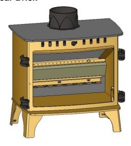
Pull the top edge of the Rear Brick towards you, lift and remove.
