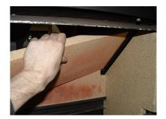
Lift the Baffle Brick and slide to the right. When the left side of the Brick clears the Baffle Support, lower the Brick into the Fire Box and remove.
