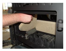
Remove all of the Riddling bars. Slide the front of the Side Brick towards the centre of the Stove and remove the Side Brick.
