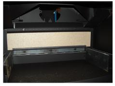
Pull the top edge of the Rear Brick towards you, lift and remove.
