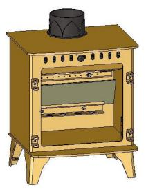
Pull the top edge of the Rear Brick forward and lift out of the Stove.
