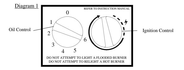
2) As soon as the burner is lit turn the oil control to position 1.
