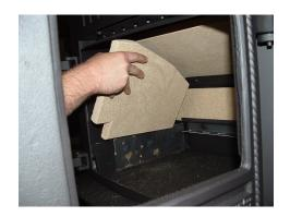
Remove all of the Riddling bars. Lift the side brick out of the groove in the side plate.
