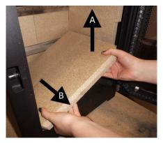
Remove the both the side bricks, taking care not to disturb the top rear bricks.
