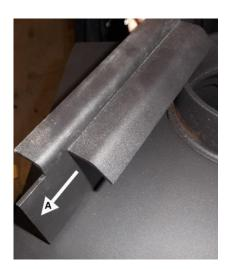
4) Offer the side plate into the stove (B), with (A) fitting into the front grate support and slide into place.
