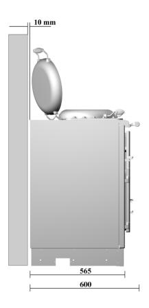
The cooker weighs 200kg and so the floor must be capable of withstanding the load. The cooker stands 900mm high and so will be the same height as standard kitchen units without the use of a plinth. If the floor is not level the cooker should be made level with the use of packing pieces. The cooker does not require access via the side panels once it is installed and so kitchen units can be butted up to the sides of the cooker.
