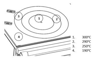
Figure 14 Approx. Working Temps 30 Mins. After Refuelling
