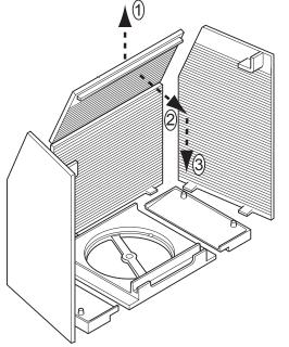
The upper protection plate is held in place by the two side protection plates. To remove (1) lift up the plate and then (2) draw it towards the front of the fire box.
