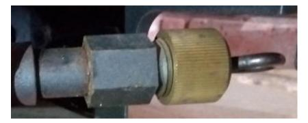
Every two weeks, if running a lot, or once a month, if not, undo the knurled nut half a turn, pull out the rod straight back then push it in turning it to clear any carbon out and this pushes it into the burner. This keeps the oil flowing well into the burner.
