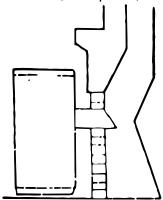
3. Technique used when chimney needs lining or part lining. Fire opening sealed as in I or 2 with healer spigot connected to asbestos or steel Tee. Flue lining connected to one arm of Tee. Bottom arm left open to permit debris to fall without blocking heater spigot.
