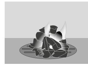
If the fuel is manufactured smokeless coal the air direction lever should remain in the mid position. If the fuel is anthracite the lever should be set to its lowest position. Whichever coal is being used the air volume should now be set to the 12'O clock position.
