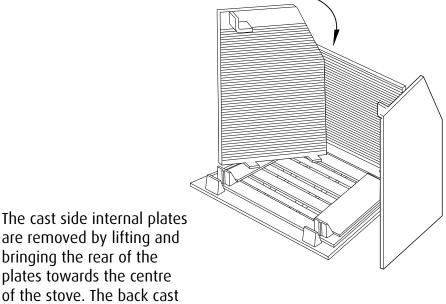
plate is removed by pulling the top towards the front of the stove.
