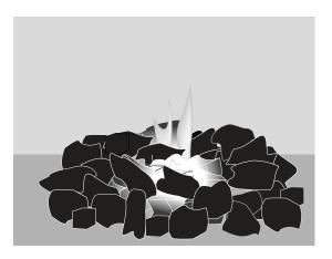
New loading of coal should be placed to cover only coals which are glowing. It will delay the ignition of coal not already burning if further layers of coal are added to them. Smoke production will be reduced if new coals are added only when the coal has stopped emitting flames but is glowing brightly.
