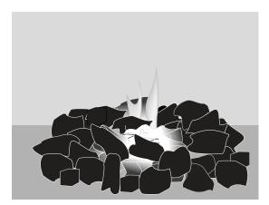
New loading of smokeless coal should be placed to cover only coals which are glowing. It will delay the ignition of coal not already burning if further layers of coal are added to them. Smoke production will be reduced if new coals are added only when the coal has stopped emitting flames but is glowing brightly.
