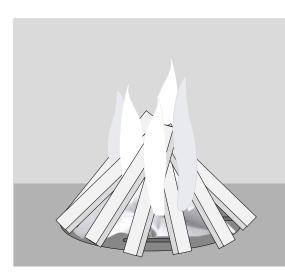
The kindling wood should be placed over the paper so as to rest against each other in a conical formation, leaving space between each piece.
