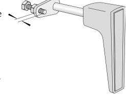
To adjust the furnace door handle latch, loosen the locking nut and adjust the bolt as required. Retighten the locking nut. The adjustment should be made so that when the handle is in its closed position the door is air tight.
