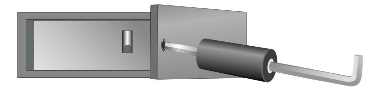
The stove tool right angle end is used to engage the ash pan socket. Care should be taken to ensure the tool is fully engaged before removing the ash pan. The glove should always be worn on the hand not operating the stove tool so that the ash pan can be securely held. Do not put the ash into, or with, anything combustible; even seemingly cold ashes may contain small glowing embers capable of igniting items they come in contact with.
