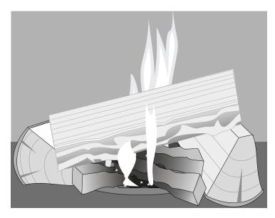
When the previous loading of wood is burning brightly add another log to bridge the fire. Always avoid putting wood directly onto wood burning with flame because the new, cold, log will tend to cool the flame giving gasses below their ignition temperature.
