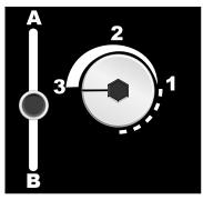
When the direction lever is in its uppermost position the air enters the stove above the fire, and when set to its lower position air enters the stove from beneath the grate. Positioning the lever at its mid position will supply air both over and under the fire and this position is used when lighting a fire or burning manufactured smokeless coals. It should be set to its bottom position when burning natural smokeless coal such as anthracite and at its top position when burning wood.
