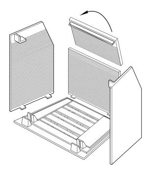
For stoves other than the 43 models the sloping cast back plate is removed by lifting upwards and towards the front of the stove.
