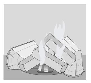
Wearing the stove glove open the door and place a log to either side of the burning kindling and larger than kindling wood over, but not smothering, the kindling.
