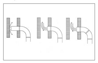
In order to maintain the temperature in a flue any external flueing must be of twin wall constructions.
