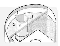
If required for installation, the stove pod shelf can bear a static load of up to 56kg
