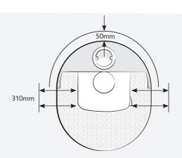
The unshielded sides of the Aire 3 must be positioned a minimum of 310mm from combustible material in accordance with the Installation manual supplied with the Aire 3. The stove pod base allows the stove pod with the Aire 3 on it to be placed on any hard / flat surface and does not require an additional hearth underneath it.
