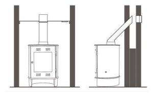
Attach the flue outlet to the stove with the screws and nuts provided. Use a steel closure. Attach the flue outlet to the stove with the screws and nuts provided. Use a steel closure plate to seal off the chimney; a cleaning door must be fitted into the plate or flue, and a steel sealing collar must be used to fit the flue into the steel plate. Seal all joins with fire cement.
