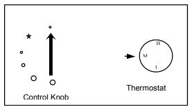
setting and the fire will light. To turn the fire off, rotate knob fully clockwise.
