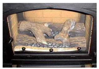
The base and front logs are fixed in position and should only need removing for servicing. The base log locates onto the burner and the front log is pushed to the extreme left hand side. Take the 2 loose logs\* and position them as shown onto the cut outs on the base log, taking care to locate them correctly to ensure clean combustion. No additional logs should be added to the fire.
