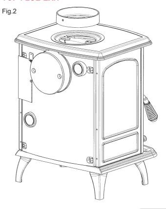
For the top outlet configuration, remove the blanking plate from the hob, remove the flue spigot from the back plate and fix it to the hob. Fix the outlet blanking plate to back plate (see Fig. 2). Push the flue outlet connector pipe (not supplied) into the flue spigot and cement into place using approved fire cement, ensuring that no cement is blocking the flue passageway.
