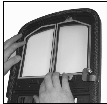
Fig. 6 Lining up the gasket
