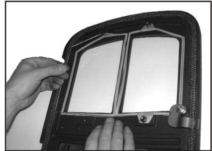
Fig. 7 Fitting door glass
