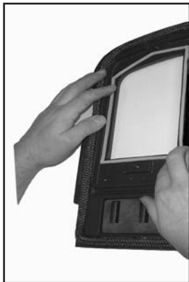
Fig. 6 Lining up the gasket
