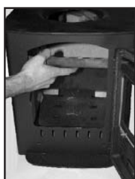
Fig. 2 Inserting throat plate
