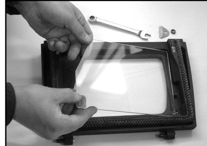
Fig 6b fitting new glass
