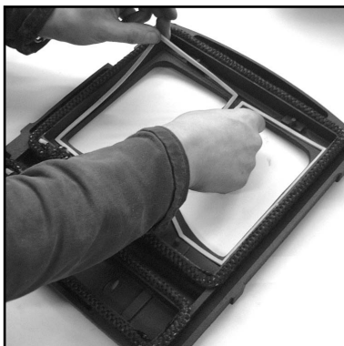
Fig. 6a fitting new door gasket (Hamlet Hero Shown)
