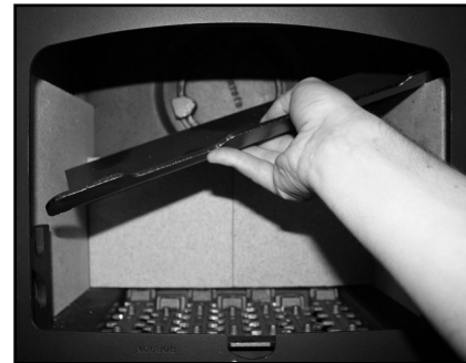
Fig. 11. Inserting the throat plate
