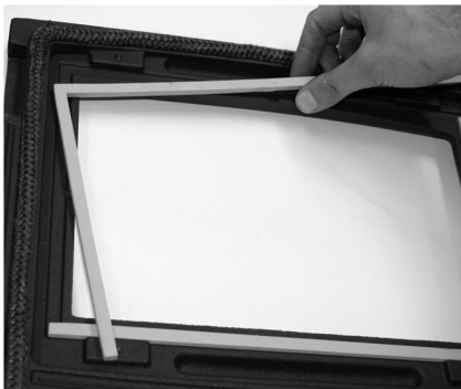
Fig. 17. Lining up the gasket
