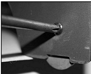
Fig. 4. Adjusting the rear feet
