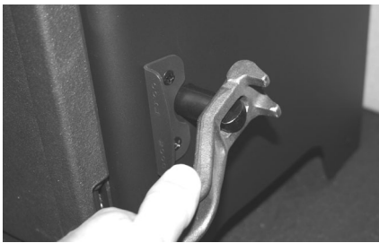
Fig. 24 Setting The Grate
