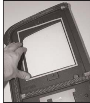
Fig. 6 Lining up the gasket
