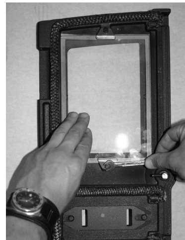
Fig. 18. Tightening the glass clips
