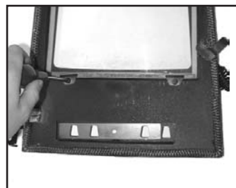
Fig. 6a Unscrewing glass clips.
