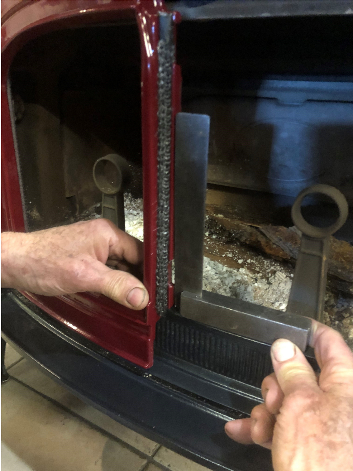
Figure 8 Check the vertical alignment of the door.
