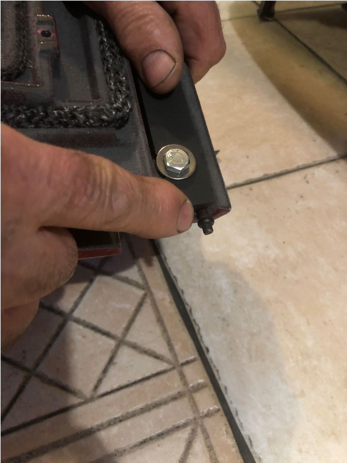
Figure 5 Set 12 mm to bottom of hinge pin and tap back to 10mm.
