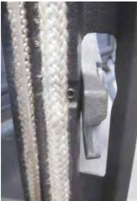
Grub screw visible to the side of the door handle on some models
