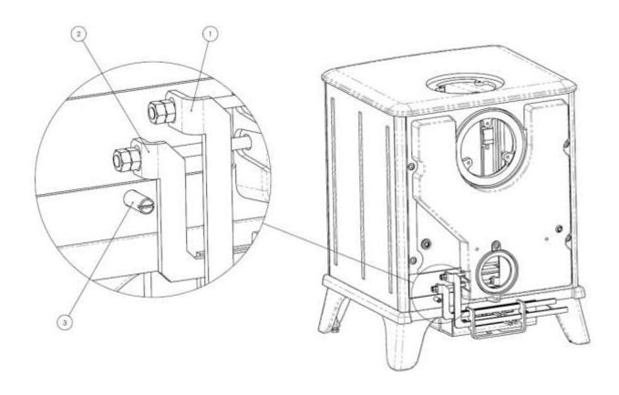
If the stove is being installed into a property which is not in a smoke control zone, you can simply screw the threaded rod into the stove (this will allow the slider to fully close and cut off the air supply)
