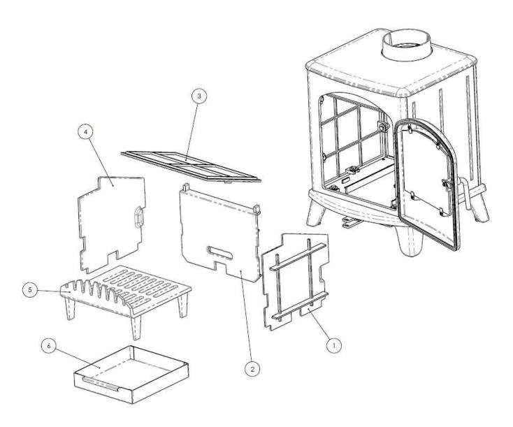
To refit the internals follow the numbered sequence from 1 - 6. The firebricks should fit quite snug however small gaps are acceptable due to cast iron tolerances. Be careful not to trap or squash fingers at this stage.
