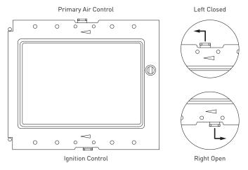
The primary air control regulates the air to your fire for desired combustion rates and to keep your fire window clear.
