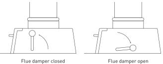
Opening the flue damper will allow heat to pass directly to the chimney via the left side of the hotplate, useful for boosting the hotplate temperature without increasing the main oven temperature.
