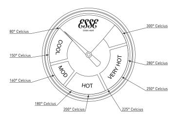
The temperature dial on the main oven door provides an indication of the oven temperature and by comparison the temperature of the adjacent ovens.
