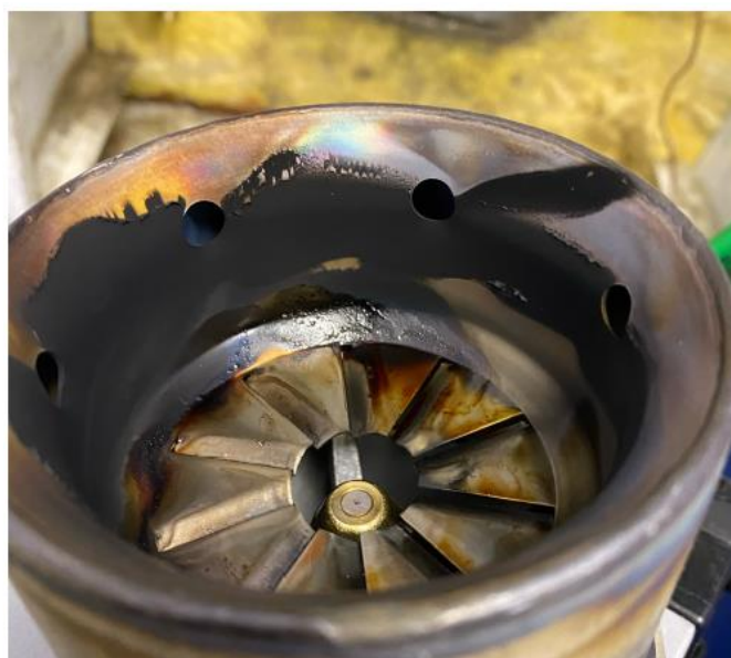
Figure 15: Carbon deposit build-up on the blast tube of an incorrectly converted burner
