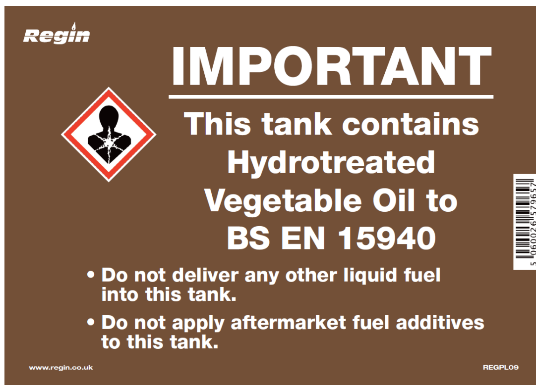
Figure 5: Example tank storage safety label for HVO
